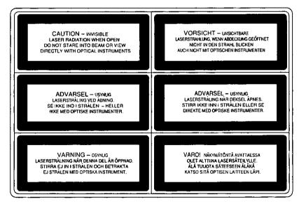
• This label is attached to the bottom of the drive unit.
