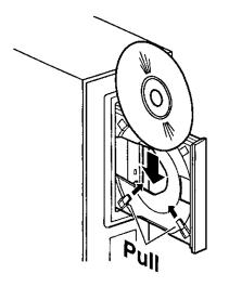
There are four disc clips that will hold a disc in place vertically on the CD-ROM drive tray When you install the CD-ROM drive vertically, please pull the two disc clips near the bottom edge of the disc tray and load a disc vertically as left figure 5
